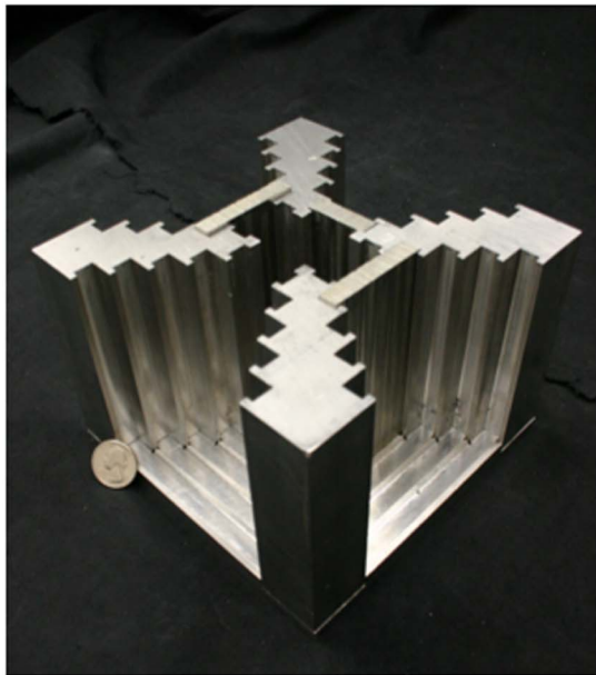
FIG. 2. (a) The M^3R shielding aperture and base with three pinhole plates in place. Cameras abut each of the four ports and a lid locks onto the top of the assembly. (b) A top view of the shielding assembly design. Example pinhole plates are shown on the left side of the figure and a representation of a gamma camera is shown at each port. Distances given are in inches.
