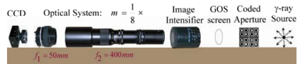
Fig. 3. An exploded view of the prototype gamma-ray microscope.
