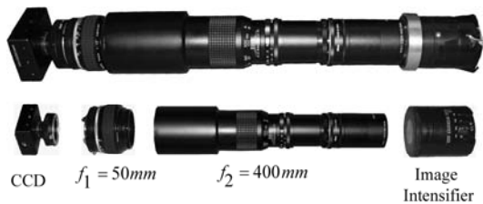
Fig. 1. BazookaSPECT gamma camera in an 8:1 imaging configuration.
